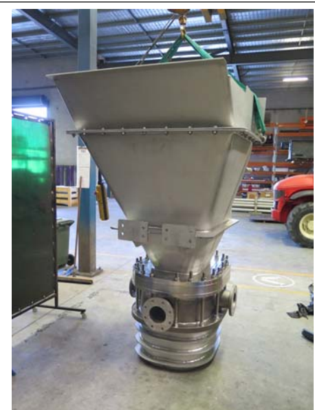
Induced Draft feed port prior to installation
